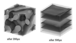
Time evolution of PAN-b-PS system. The boundary between PAN and PS regions is represented with isosurfaces. In dark grey is represented PS.
