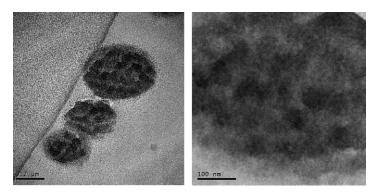
**Figure 8.**TEM images of nanospheres of PAN-*b*-PS system cutted and shadowed with RuO<sub>4</sub>, revealing the inner organization (images kindly given by Massimo Lazzari, University of Santiago de Compostela, Spain.)
